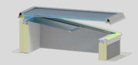
MULTIFILM® sun and glare protection system. Cross section
